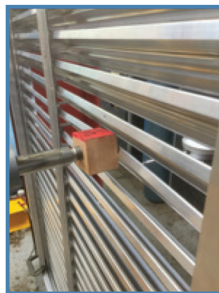
Point Load (Internal View of Test)
